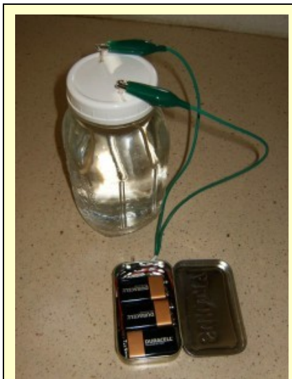
A homemade 27 volt colloidal silver generator. We recommend not bothering to do this.
